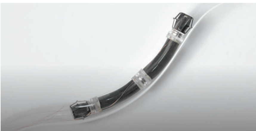
Worm-inspired robot for centimeter-scale pipeline inspection. (PHOTO: SCREENSHOT)
