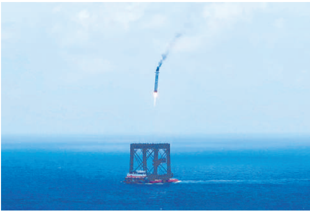
The offshore recovery platform successfully recovered the first stage of the Long March-10B carrier rocket using the net-capture method on July 10, 2026. (PHOTO: XINHUA)
