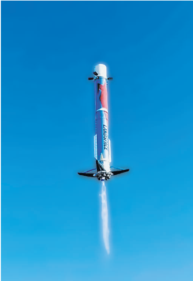
China launches its reusable rocket Zhuque-3 Y2 on August 19, and achieves its first successful land-based controlled recovery of a rocket's first stage using deployable landing legs. (PHOTO: XINHUA)
